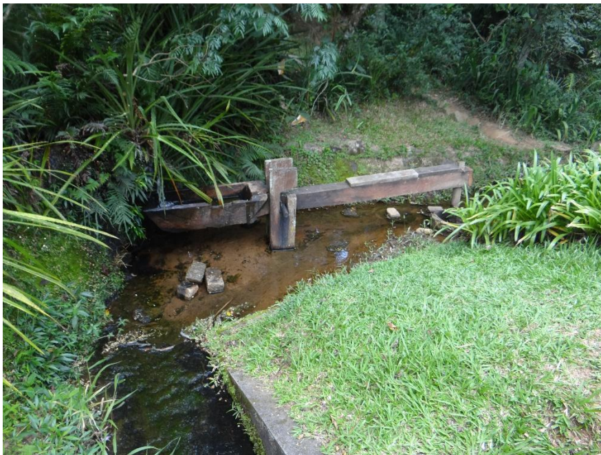
The Hammer Water Wheel (Monjolo) Photo: RT Shirasuna
